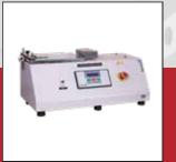
Coefficient of Friction Tester
